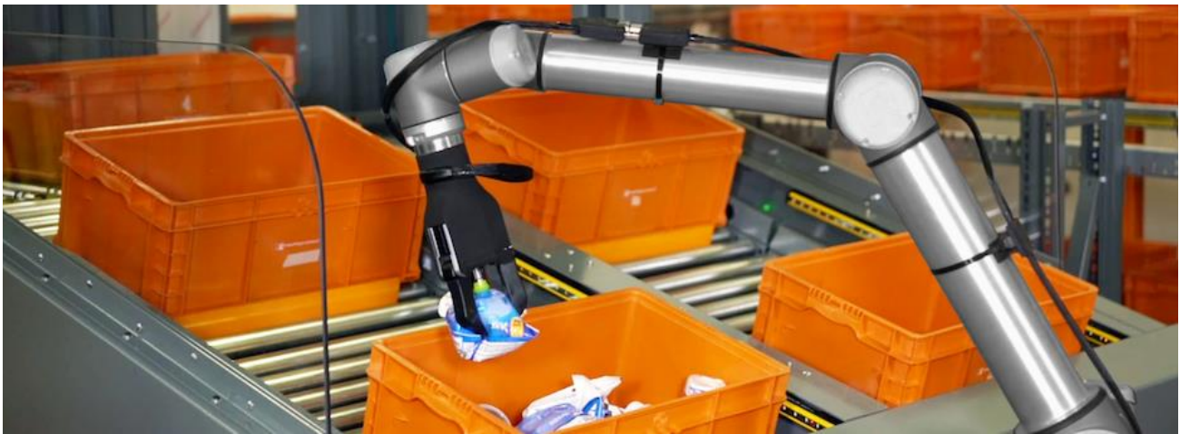
Exhibit 18 Startup RightHand Robotics Uses a Combination of a Suction Cup and "Fingers" to Handle Diverse Item-Picking
