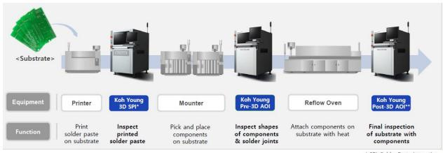
\* SPI: Solder Paste Inspection \*\* AOI: Automated Optical Inspection
