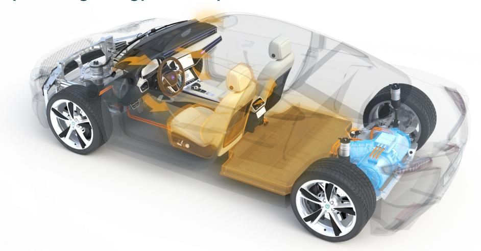
In order to optimize energy while increasing the All Electric Range, a perfect thermal management system is key. Ideal performance of the battery requires a temperature between 20-40°C. Without the free heat of a classical ICE, the energy for heating & cooling the cabin needs to be optimized.
