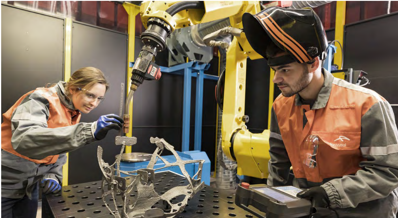
Final inspection of part made by wire and arc additive manufacturing
