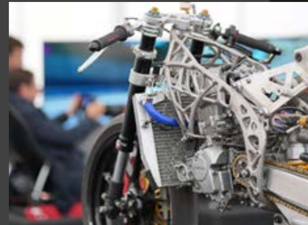
Lightweight steel motorbike chassis ↑ with 3D printing technology
